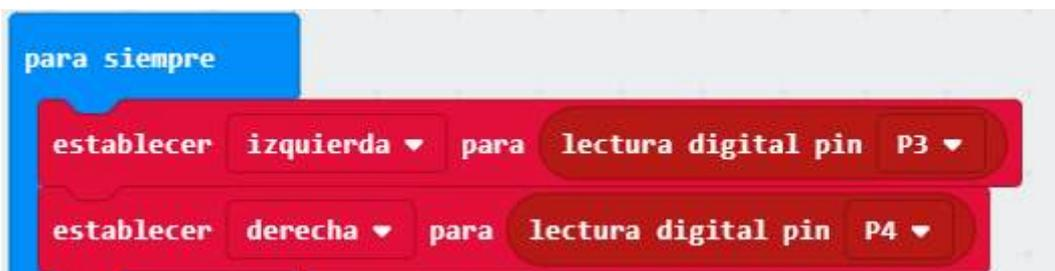
The screenshot shows a Scratch code block starting with a blue 'para siempre' (forever) loop. Inside the loop, there are two red 'establecer' (set) blocks. The first block is 'establecer izquierda' para 'lectura digital pin' (P3). The second block is 'establecer derecha' para 'lectura digital pin' (P4).
