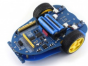
Mobile robot development platform, compatible with Raspberry Pi/Arduino
