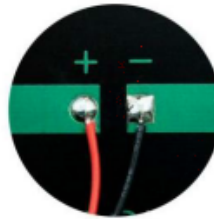
Welded wires for power supply
