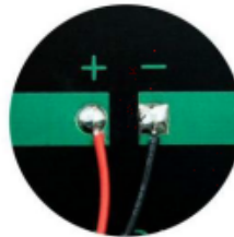
Welded wires for power supply
